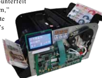
Multi-spectral image based counterfeit banknote detecting system
