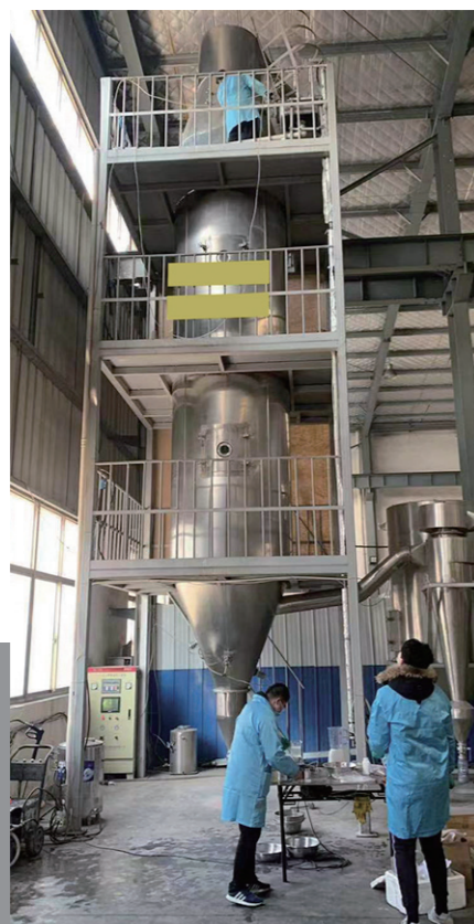
Pressurizing a perovskite oxide liquid slurry and adjusting the spray-drying temperature in the above device produced particles at a useful size.
