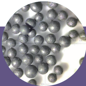
A perovskite oxygen carrier material developed by a Tsinghua team in 2021, after calcination.
